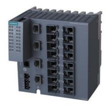
SCALANCE XC216-4C G (E/IP) managed Layer 2 IE switch; IEC 62443-4-2 certified; Full Gigabit; 12x 10/100/1000 Mbps RJ45 ports; 4x 1000 Mbps combo ports (either 1000 Mbps/ SFPs or 10/100/1000 Mbps RJ45 ports can be used); 1x console port; diagnostics LED; redundant power supply; temp. range -40 °C to +70 °C; mounting: DIN rail/S7 mounting rail/wall; redundancy functions; Office features (RSTP, VLAN,...); PROFINET IO device; Ethernet/IP-compliant; C-plug slot; Default EtherNet/IP
